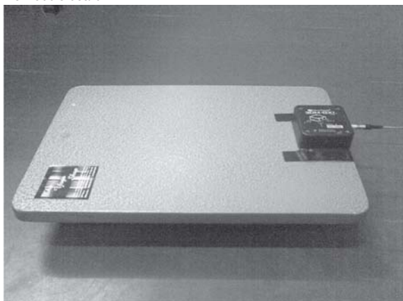
Fig. 2: Wobble Board Top Surface. The IMU is attached to the top surface of the wobble board.
